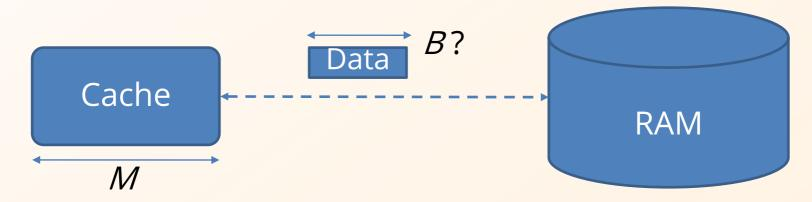
Analýsis for 2-level memory is applicable for unknown multilevel memory (register, L1C, L2C, ..., LLC, memory).
