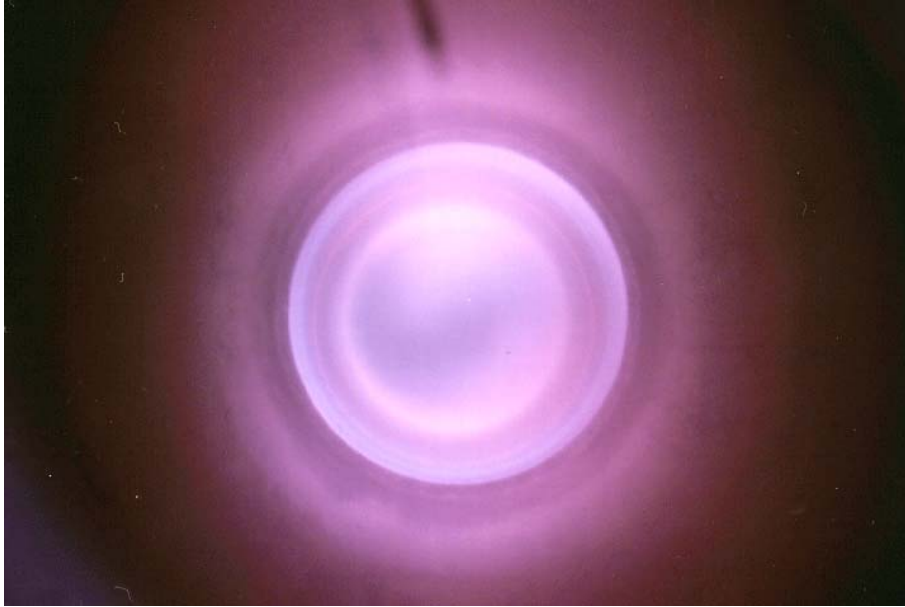
Figure 6.1: Typical light intensity of the argon plasma. View through the axial port.
