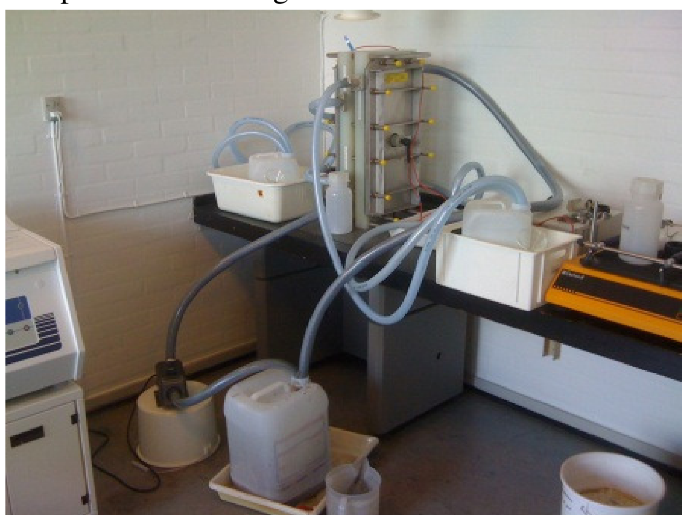
Figure 2: Electrochemical stack for pilot scale testing
